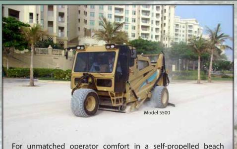
For unmatched operator comfort in a self-propelled beach cleaner, ask about the Cherrington Model 5500 Beach Screener with cab and air conditioning.
