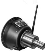
SP-IL Series SAE #1 thru SAE #0 SAE 14" thru SAE 18" Double & triple organic drive plate Capacity from 2197 to 10,170 Nm (1620 to 7500 lb.ft.) Sintered iron available In-line applications only - no side load
