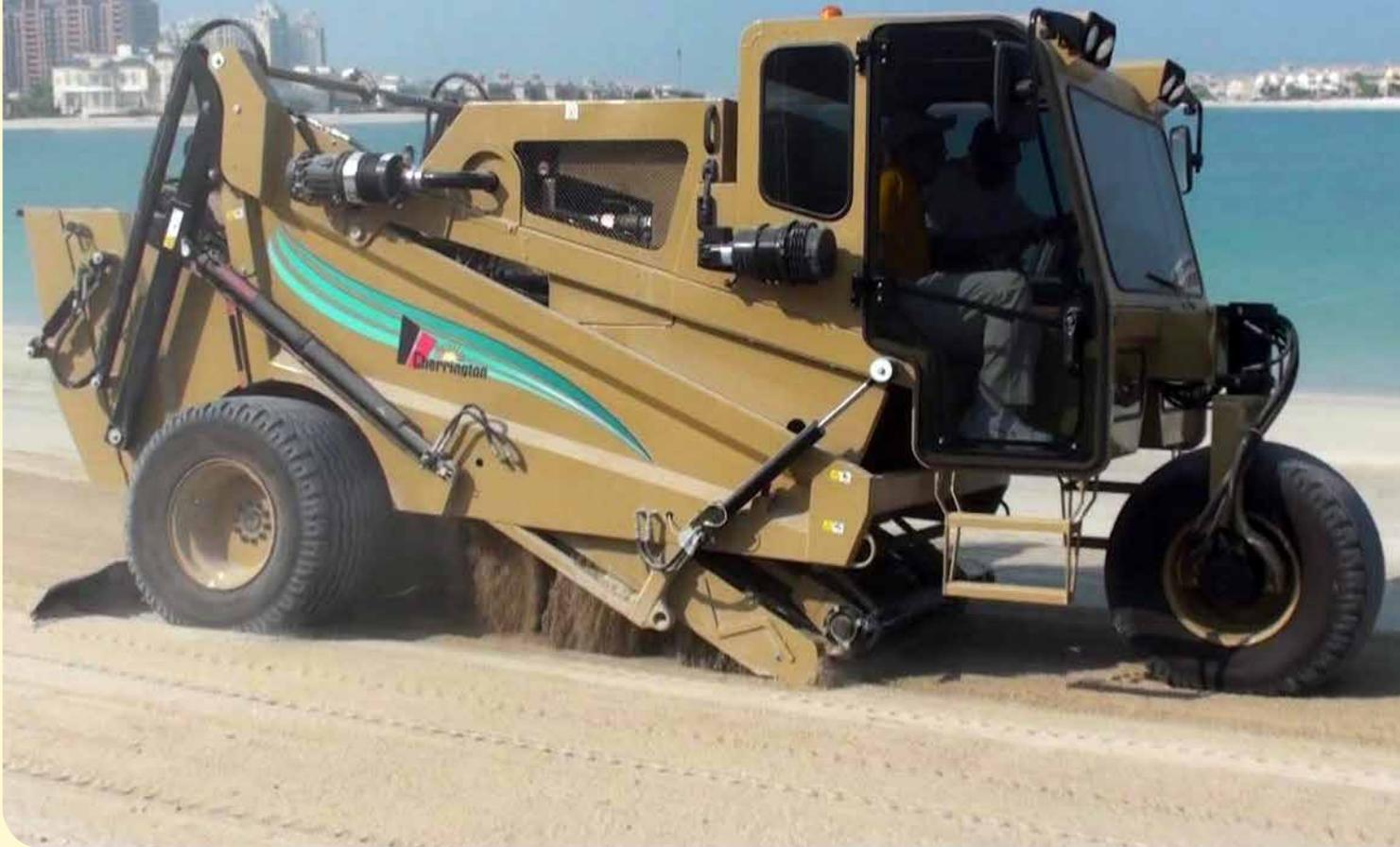
We have combined the proven isolator Lift and Screen Method with state of the art technology and modern, innovative design to bring you the new Model 5500 Beach Cleaner.
