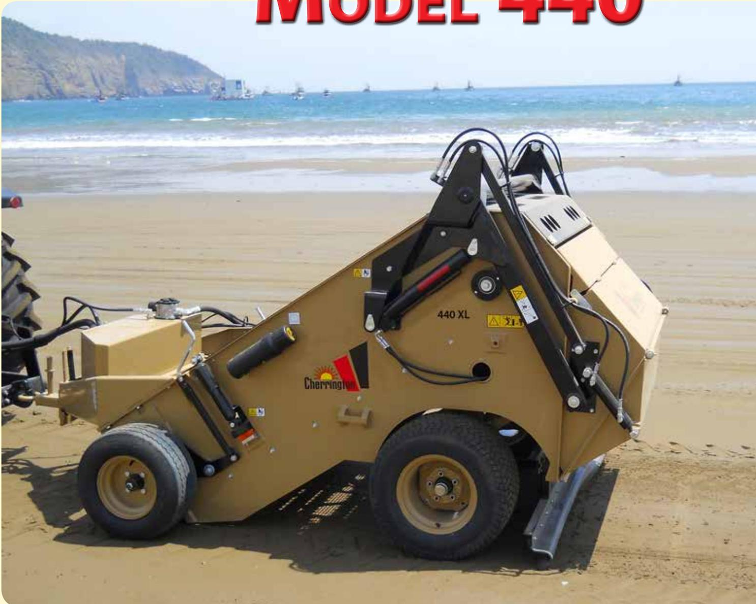
Cherrington lifts and screens the sand to screen-clean and sanitize your beach. Efficient and economical Beachcleaning using Cherrington Beach Cleaners is accomplished by lifting the sand from the beach, screening it through a powered oscillating screen, retaining all objects larger than the chosen screen size and then returning the sand to the beach.
