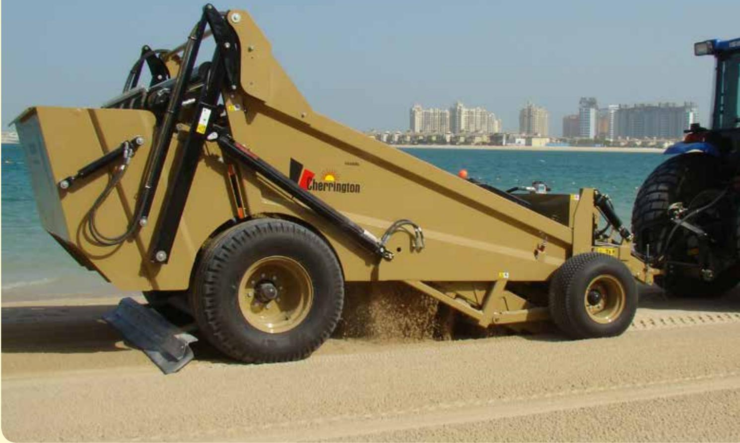
The Cherrington 4600XL is fast, rugged and dependable with only 3 bearings on the conveyor system and no revolving belts, tines, or screens for amazingly low maintenance. A galvanized screen bed and loading paddles, high-speed stainless steel screens, and carbide glide pucks make for a long life and smooth, quiet operation.
