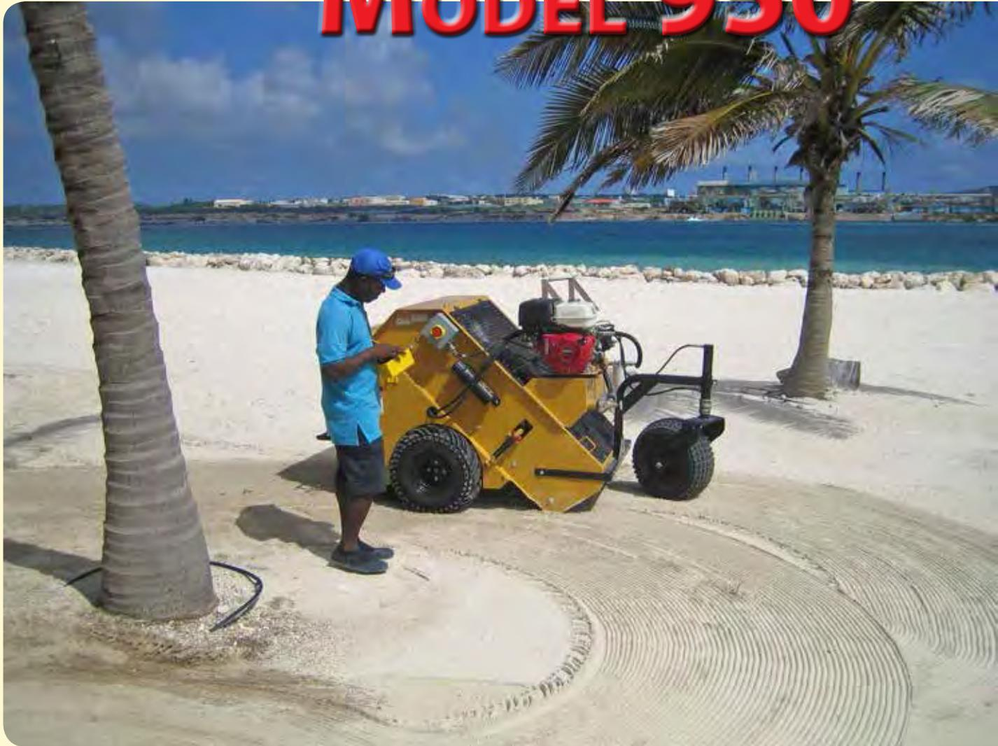
Like all Cherrington Screeners, the Model 950 efficiently collects everything larger than the selected screen-hole size. The Cherrington Model 950 is shipped with two separate interchangeable screens to allow you to adapt quickly to changing screening conditions. The  $\frac{1}{2}$ " (13mm) and  $\frac{3}{4}$ " (19mm) wire screens are standard and the  $\frac{3}{8}$ " (9mm) and 1 inch (25mm) screens are available for special screening needs.
