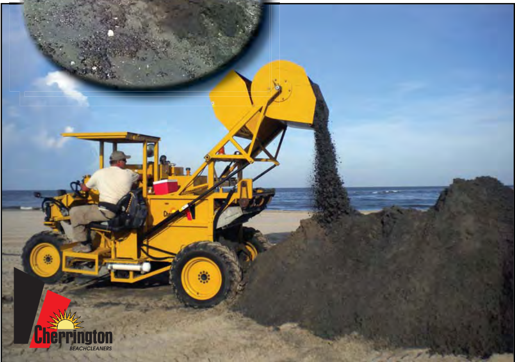
The Model 5000 skims off and loads contaminated sand and tarballs into the hopper for unloading into trucks using the 8.5 ft (2.6 m) high lift or onto the ground in piles for processing later in a sand wash system.
