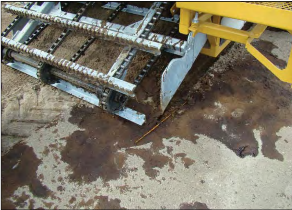
1) Digger Point With Infinite, Precise Depth Control (0-6 inches or 15cm) 3) Three-wheel Design, Zero-turn Radius for Ultimate Manueverability
