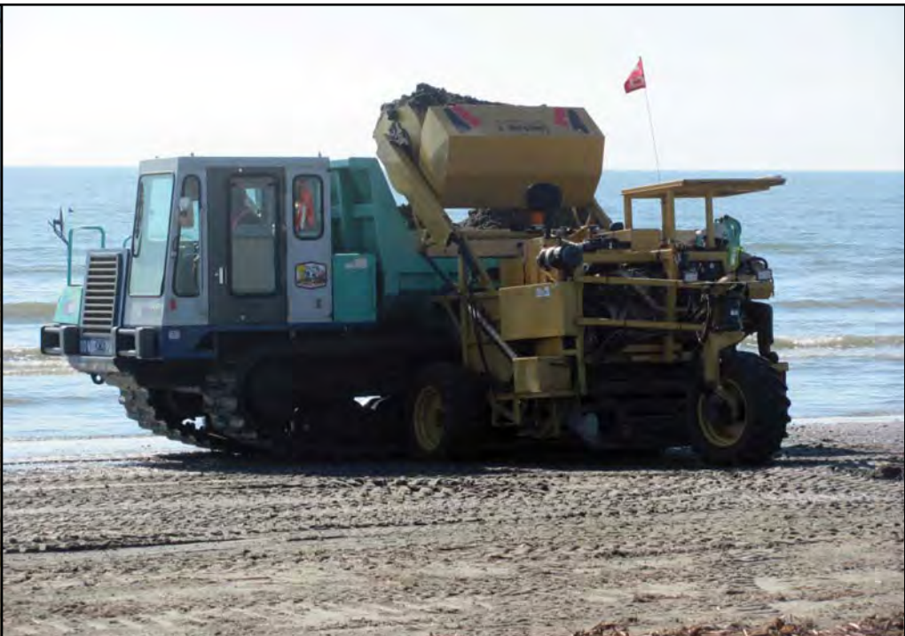
The Model 5000 skims off and loads contaminated sand and tarballs into the hopper for unloading into trucks using the 8.5 ft (2.6 m) high lift or onto the ground in piles for processing later in a sand wash system.
