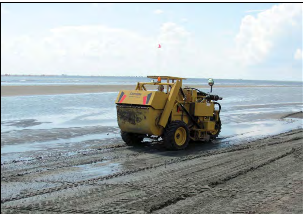
The Model 5000 skims off and loads contaminated sand and tarballs into the hopper for unloading into trucks using the 8.5 ft (2.6 m) high lift or onto the ground in piles for processing later in a sand wash system.
