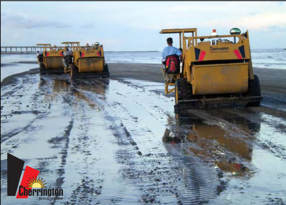
The Cherrington Model 5000's three-wheel, self-propelled design allows for excellent operator visibility of the digger point and loading paddles. The operator can quickly and easily adjust the cleaning depth as needed.
