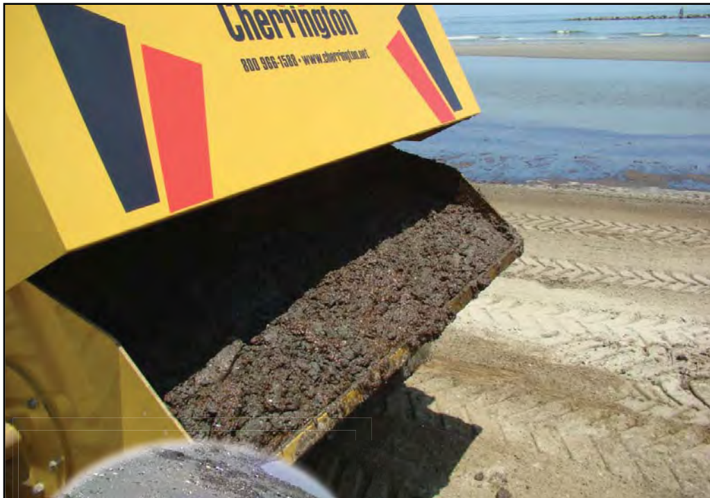
The Model 5000 skims off and loads contaminated sand and tarballs into the hopper for unloading into trucks using the 8.5 ft (2.6 m) high lift or onto the ground in piles for processing later in a sand wash system.
