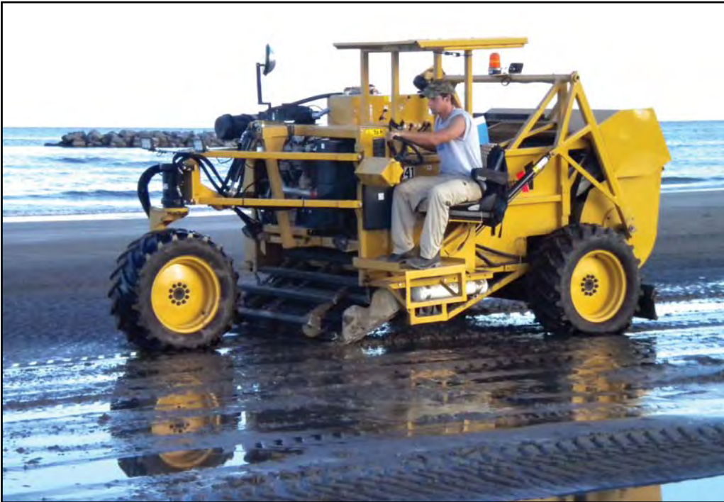
The Cherrington Model 5000's three-wheel, self-propelled design allows for excellent operator visibility of the digger point and loading paddles. The operator can quickly and easily adjust the cleaning depth as needed.
