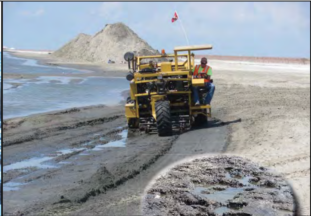
The Cherrington Model 5000's three-wheel, self-propelled design allows for excellent operator visibility of the digger point and loading paddles. The operator can quickly and easily adjust the cleaning depth as needed.
