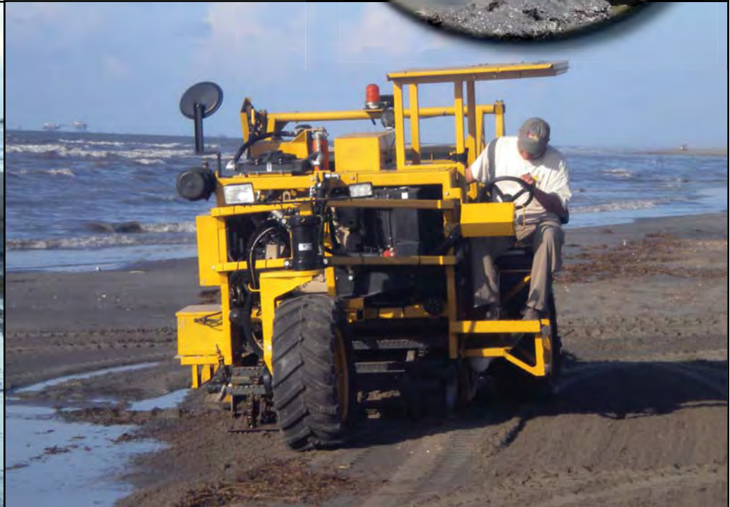
The Cherrington Model 5000's three-wheel, self-propelled design allows for excellent operator visibility of the digger point and loading paddles. The operator can quickly and easily adjust the cleaning depth as needed.
