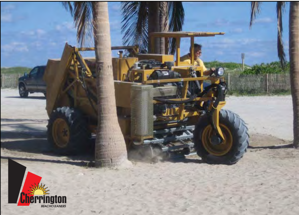
1) Digger Point With Infinite, Precise Depth Control (0-6 inches or 15cm) 3) Three-wheel Design, Zero-turn Radius for Ultimate Manueverability
