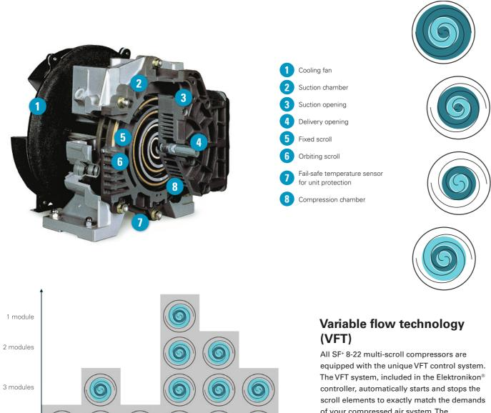
scroll elements to exactly match the demands of your compressed air system. The Elektronikon<sup>®</sup> control algorithm ensures that the system pressure is kept within a very narrow pressure band.
