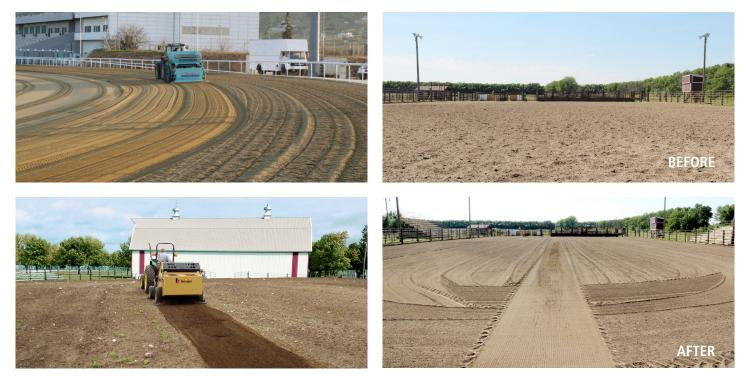
Kässbohrer Screeners will remove rocks and other debris from your arena/track all in one pass without the hassle of loading and hauling it to stationary screening plant.
