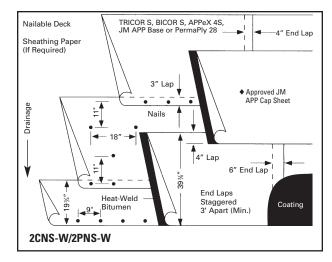
the same manner, with 4" (102 mm) side and 6" (152 mm) end laps over the preceding sheets. All laps must be rolled with a 3" (76 mm) rounded edge roller. A  $\frac{1}{6}$ " to  $\frac{3}{6}$ " (3 mm to 10 mm) bleedout of APP compound shall be visible at the edge of all seams. All laps must be checked for good adhesion.
