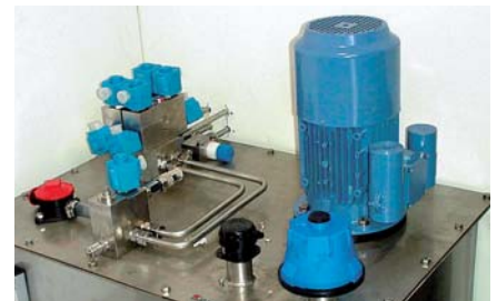
Central water hydraulic power pack.
