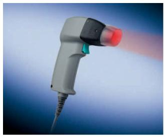
The SIMATIC HawkEye 50T and SIMATIC HawkEye 51T are high-performance, high resolution readers for low-contrast two dimensional (2D) Data Matrix direct part marks (DPMs). They incorporate advanced video image processing and illumination technology to read symbols on a variety of surfaces that have been created by dot peen, laser, or inkjet.
