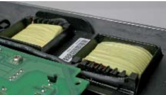
DC coils reduce harmonic noise and protect the drive.
