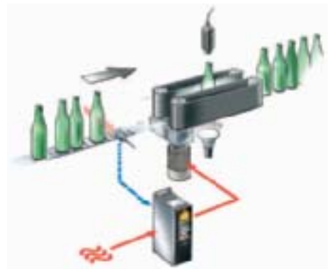
The bottle is beneath the inspection camera at the exact moment the flash is activated. The VLT AutomationDrive ensures that production speed is adapted, even in complex operations along the entire production line.
