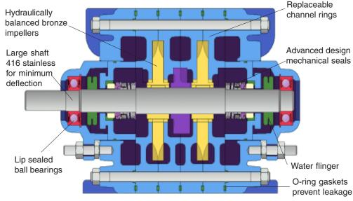
**Bearingings.** Heavy duty sealed ball bearings on inboard and outboard ends of the shaft are permanently lubricated for maintenance free service.
