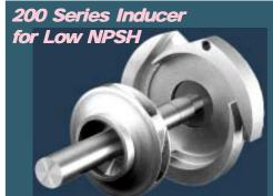
The 200 Series inducer style pumps are ideally suited to applications where available NPSH at the pump inlet is limited, such as boiler feed water deaerator service.
