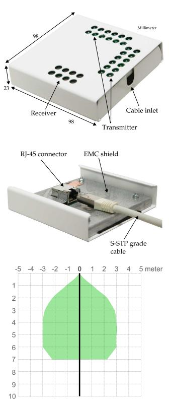
Operating range is equipment dependent. The figure above shows a radiation diagram together with the DU-111-02 Delegate Unit where the horizontal axis shows radiation diameter at ceiling heights up to seven metres.
