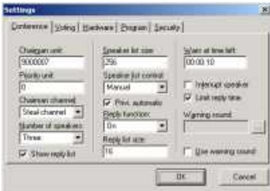
Includes and extends all *Central Unit* functionality. Adds powerful database functionality including delegate and seating lists. Speaking time can be limited automatically on individual basis using the delegate list. Separate program window displays speaker lists and voting results, suitable for video projection.
