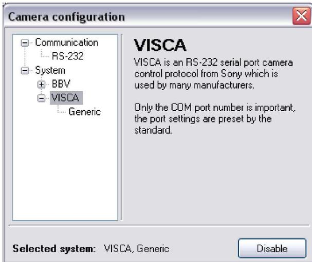
Fig. 2: Camera configuration panel
