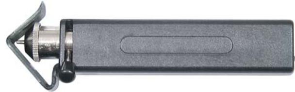
Cuts around cable jacket, slits the length of jacket for easy removal. Single or multiple conductor cable from 3/16" to 1" overall diameter. **ST-305:** Same as above, but for 1" to 1 1/2" overall diameter cables.
