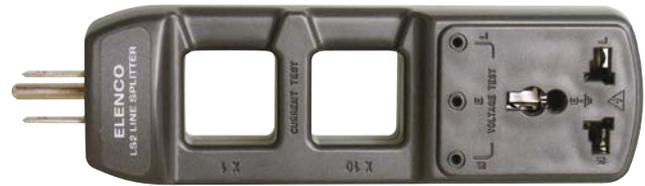
For measuring current in plug-in appliances and air conditioners. Splits two conductor line cord for reading at outlets under load. Permits voltage measurements at outlet under active conditions. Direct and 10X sensitivity.
