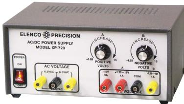
Model **XP-720K** has 3 fully regulated DC supply outputs, two outputs are continuously variable and one is fixed, plus a 12.6VAC output center-tapped to 6.3VAC.
