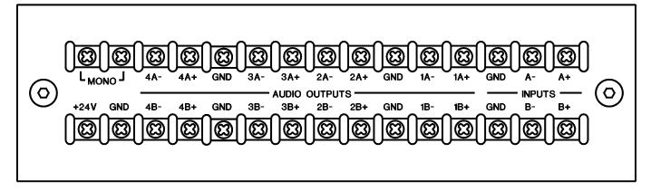
**AUDIO INPUTS:** Connect **Channel A** balanced audio to **A+**, **A-**, and **GND**. Connect **Channel B** unbalanced audio to **B+** and **GND**; connect **B-** to **GND**. If unit is being used for stereo, connect **Channel B** similarly to **A**.
