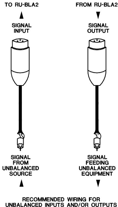
**AUDIO INPUTS:** The + and - balanced audio signals enter the unit through the front panel XLR connectors. Unbalanced audio may be connected to the + terminal, with the unbalanced shield connected to both the - and ground terminal (Pin 1).
