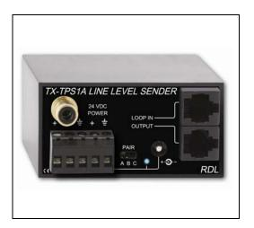
The TX-TPS1A is a single-pair audio sending module compatible with RDL Format-A twisted pair products. It is built in the versatile Max-TX series enclosure. The durable adhesives provided with the TX-TPS1A permit permanent or removable mounting. The TX-TPS1A may be rack or surface mounted with optional TX™ series accessories.
