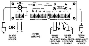
EACH INPUT MAY BE WIRED BALANCED OR UNBALANCED
