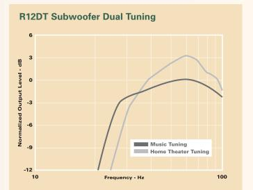
When both ports are open, frequency response allows maximum bass impact for home theater; when tuned with the supplied insert, frequency response is more accurate for music listening.
