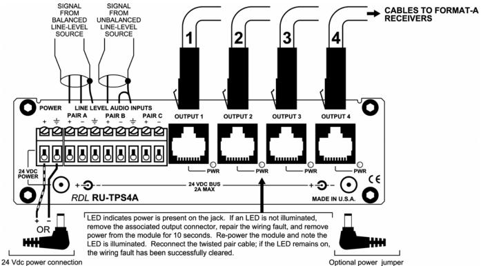
Note: Power connection is required; module may not be powered through twisted pair cables.
