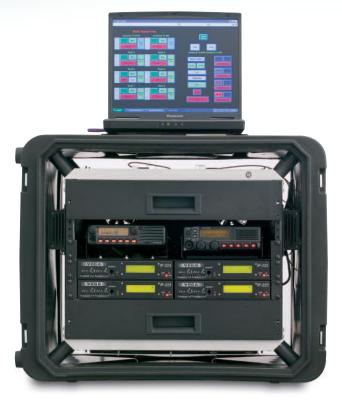
The idea behind V.I.P.E.R. is a fairly simple one. By using our innovative VoIP technology, the radio's transmissions and control information are converted into digital data—regardless of frequency or standard, VHF. UHF or 800MhZ.
