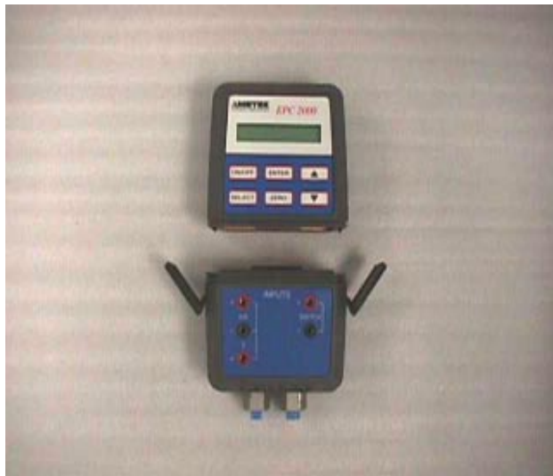
EPC 2000 Electronic Pressure Calibrator Showing Removeable Transducer Modules
