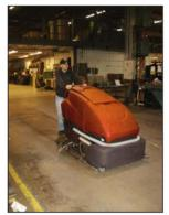
Safety and Technology The Phoenix 30 & 34 are equipped with a "belly bar" that prevents the operator from being pinned behind the machine when in reverse mode. Also standard, is a color coded LED battery gauge that will let the operator know if any error code faults are coming from the on-board computer. This helps pinpoint any problem for guick and easy repair.
