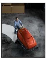
Durable Construction The Phoenix 30 & 34 are made with a powder coated, epoxy painted, 11 gauge steel frame to resist corrosion. The tanks and bumper are constructed of a heavy-duty rotationally molded polyethylene. Rugged construction and reliability, a PowerBoss "hallmark", means that the Phoenix 30 & 34 scrubbers are built to last.
