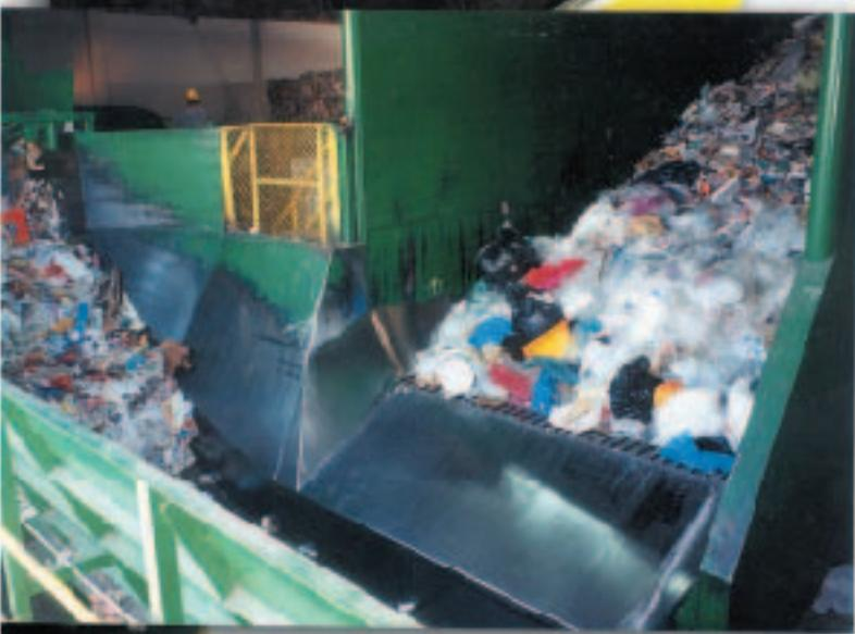
After recyclables are removed from the waste stream, materials are collected in sort bins directly below the picking lines. Suitable for nearly any material, *WALKING FLOOR* bins provide multiple options for storing, routing and sorting incoming material.
