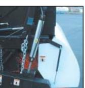
To assure contour sweeping, the cylinder lowers with no resistance. This allows the main broom to follow road contours seamlessly. The broom is driven by a hydraulic motor via an efficient chain drive system.
