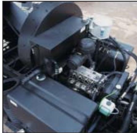
To maintain a clean supply of intake air, the A4000 is outfitted with a 2-stage, dry-type air filter that includes a Sy-Klone<sup>®</sup> centrifugal precleaner. A three-point automatic shutdown system eliminates the potential for engine damage due to high coolant temperature, low coolant level or low oil pressure. These features help ensure a long service life for the A4000’s auxiliary engine.
