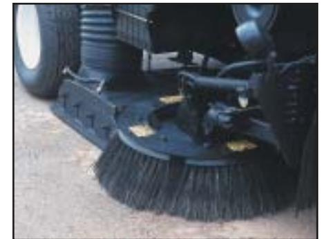
Schwarze’s industry-leading *Gutter Broom Extension Override*<sup>SM</sup> (*GEO*<sup>SM</sup>) system enables the brooms to scrub directly in front of the head.
