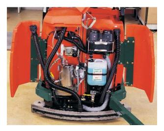
Direct access to all important parts and systems thanks to covers which can be opened for service and maintenance purposes. Pictured above for example, chemical metering system and dirty water recycling system.
