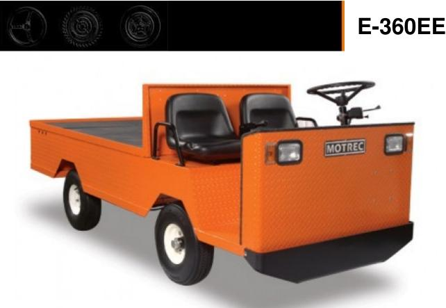
The E-360EE burden carrier is a UL Approved Type EE Powered Industrial Truck.
