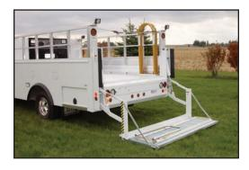
Stellar's EDL-16-86 1600-pound all-hydraulic liftgate with a galvanized grip-strut platform and folding rail tire stop is optional. Top mounted brake, turn, and marker lights are used for greater visibility and safety and are standard equipment.
