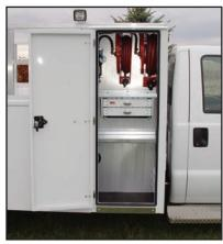
Twenty-six-inch wide front vertical compartments with box extensions are standard. The available SHD-66DD direct drive hydraulic or the SGD-2040 gas powered air compressor is located top center in the truck bed. Here the compressor is protected from the elements, is easier to maintain and service, and provides for a better balanced truck.
