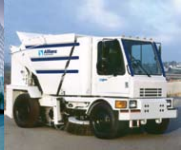
4000 Purpose Built Mechanical Four Wheel Street Sweeper.
