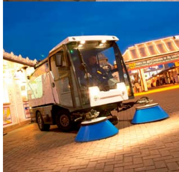
RIGHT BELOW Articulated brushes allows efficient cleaning of debris from underneath cars, benches and other obstacles.
