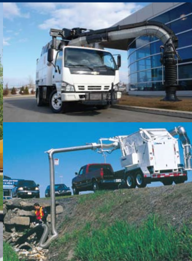
BELOW LT500: huge volume litter capacity with joystick operated robotic arm
