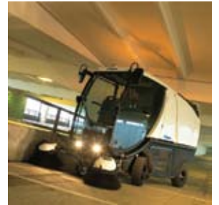
ABOVE Joystick controlled, fully articulating brushes collect hard-to-reach debris leaving a spotless path.
