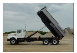
Stellar's unique A-frame tilting section allows full visibility of the lifting hook from the driver's seat during container engagement. The 52,000 pound loaders have cab mounted control levers that use the finest cables available on the market.
