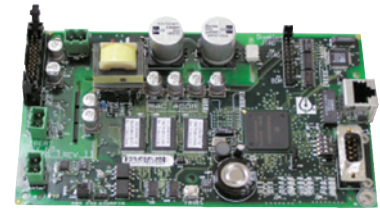
The OpenComms NIC Card transforms Liebert units into manageable nodes within your Network, NMS and BMS systems.
