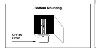
Installing the air flow switch in a horizontal duct is recommended. However, if the velocity of air flow exceeds the flow rates shown in the Vertical Duct Chart to the right, the air flow switch may be installed in a vertical duct with **upward** air flow.
