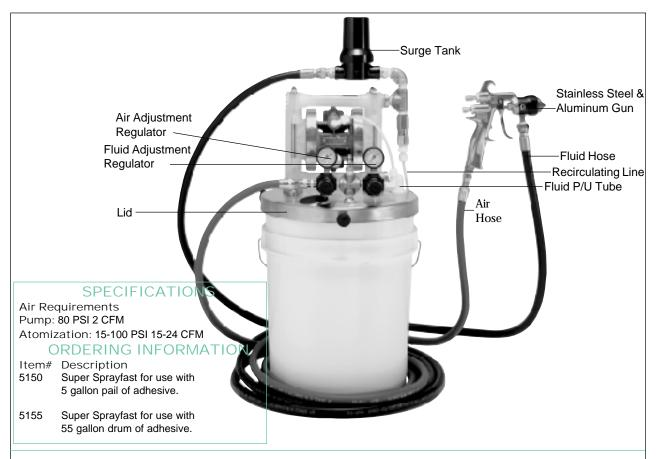
The Super Sprayfast is specifically designed for use with Duro Dyne's Water-Base Adhesives.
