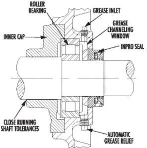
For long life and superior protection, the 661XL features the exclusive Positive Lubrication System (PLS), which channels grease directly into the bearing track. Inpro seals protect the bearings on both ends from contamination. Roller bearings on the drive end assure compliance with the API661 bearing life requirement of 40,000 hours.
