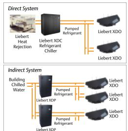
The indoor Liebert XDC refrigerant chiller is specifically designed to support Liebert XD cooling modules. The Liebert XDC connects directly to the XD modules.
