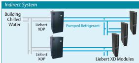
The indoor Liebert XDC Refrigerant Chiller is specifically designed to support Liebert XD cooling modules. The Liebert XDC connects directly to the XD Modules.
