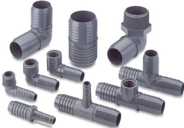
Engineered to provide positive grip and ease of installation. High quality and reliability have made Spears® insert fittings the preferred choice for irrigation and O.E.M. applications. A wide variety of PVC insert configurations and adapters are available for use with polyethylene pipe sizes 1/2" through 4", plus 6" & 8" Couplings and Adapters for lay-flat type irrigation hose. Special 3/8" barbed configurations allow clamp-free connection to 1/2" I.D. polyethylene irrigation hose.
