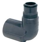
Designed for use with female acme thread O-ring seal style rotors. Provides faster installation and positive O-ring seal. Reduces the risk of over tightening and eliminates the need for thread sealants. Available as an individual component.
