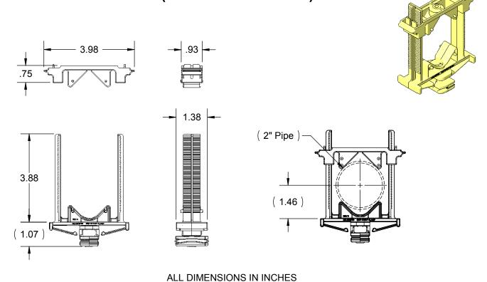
The HOLDRITE Strut Clamp™ #287-S is a fire retardant and smoke variable closure clamp. Clamp supports 1" to 2" CTS/IPS tubing sizes. Supports Copper, PEX, CPVC tubing, conduit, etc. Material meets ASTM E-84 25/50 and UL94V-0 fire rating.
