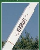
Non-Insulated Aluminum Inner Boom for increased payload and less wear and tear on chassis
