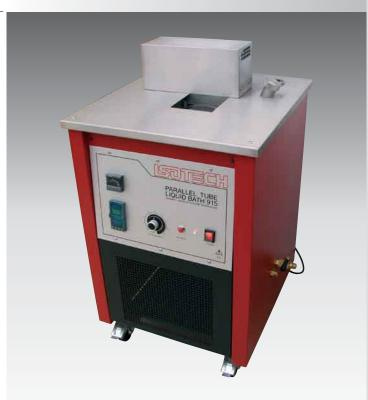
The standard temperature controller has resolution from 0.01°C to 0.1°C which auto scales to suit the four digit display (all digits can be read with the Cal NotePad Software).
