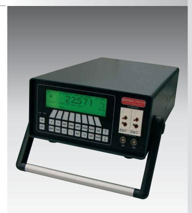
accuracy of an instrument, if you need small measurement uncertainty for high temperature PRT work you need this feature. Add the internal scanner to expand the instrument to have up to 10 channels - any or all can be scanned and lodged with the internal data logger.
