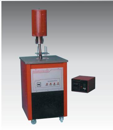
A disadvantage of many fluidized-bed baths is that good temperature stability and uniformity cannot be achieved in the fluidized medium itself. They are obtained by using large metal blocks or by inhibiting the fluidizing action in the powder around the work piece - either locally, or by completely collapsing the bed at the required temperature, this is not the case with the 875. A full evaluation report is available upon request.
