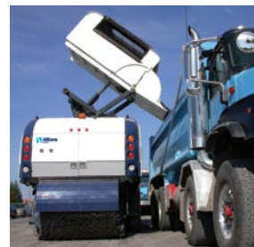
RIGHT MS350/MT350 Variable height debris dumping system from ground level up to 120 in. Optional 138 in. ultra high side dump available.
