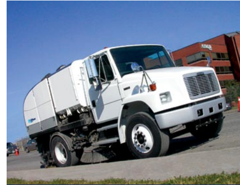
ABOVE Polyethylene water tank capacity is 375 gallons and baffled to minimize stress related movement
