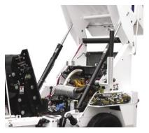
9 Low-maintenance drive system with twin wheel motor design reaches road speeds of 25 mph and handles steep grades up to 21°. No need to ride the brake to creep along for heavy sweeping- operator has smooth control at all speeds.
