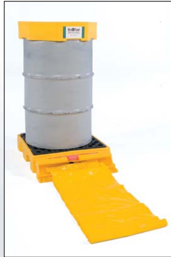
Large, catastrophic leaks flow into the bladder through a bulkhead fitting. Protective "trap door" opens automatically to allow bladder to unfurl.
