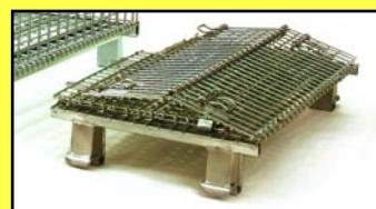
Collapses to 1/10th the original size when not in use for convenient, easy storage and handling.
